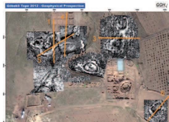
Ground penetrating radar map (timeslice 14ns) with the position of the geolectrical sections indicated (orange lines, map: GGH).
